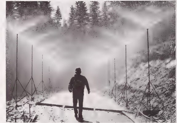
To discover how rainfall affects sediment production from forest roads, we apply an artificial rainstorm of known intensity and duration to an instrumented section of road. Later, a technician will collect sediment samples for analysis.
